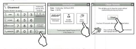
Step 4. The touch screen will be disabled for 10 seconds. Clean the bare screen or the protective film using a soft dry cloth or a cloth moistened with Isopropyl Alcohol.
